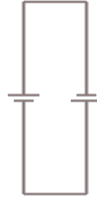
short circuit of two batteries
